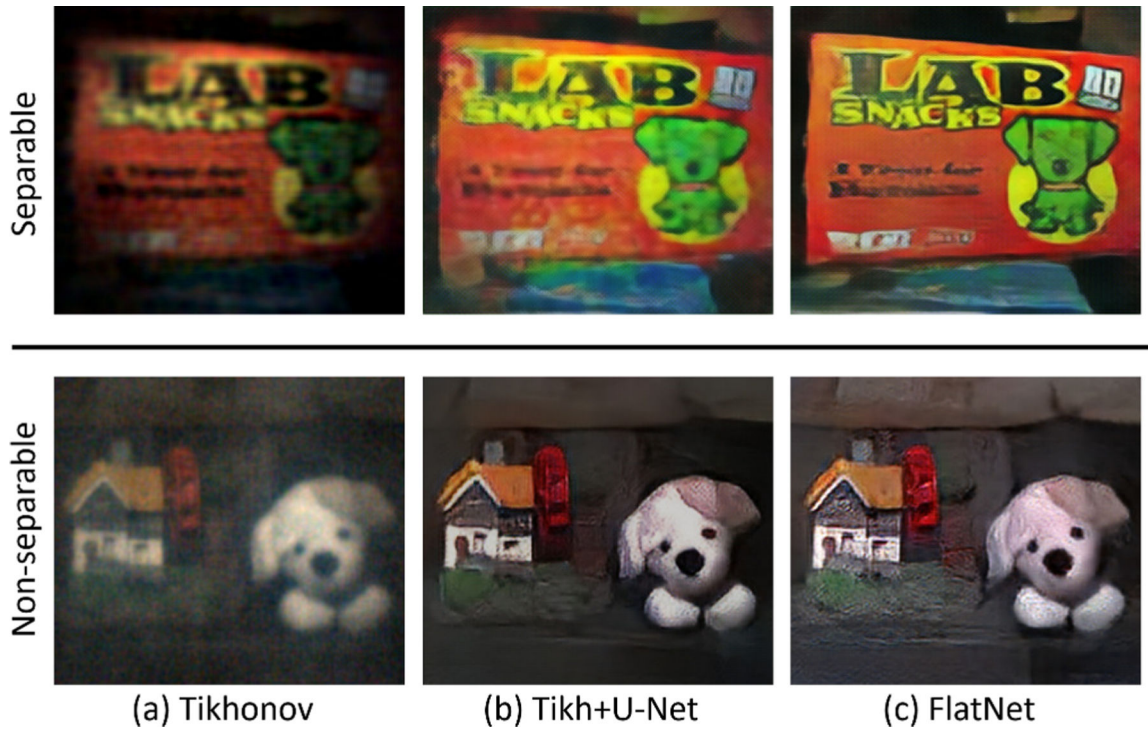
Fig. 8. Comparison of FlatNet with Tikh+U-Net.
