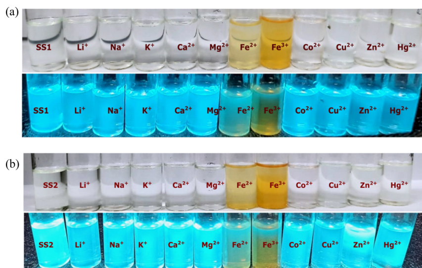
Figure 3. (a) Color changes of SS1 (10 \mu\text{M} ) with different metal ions in THF/water (7:3, v/v) solution; (b) color changes of SS2 (10 \mu\text{M} ) with different metal ions in THF/water (7:3, v/v) solution.
