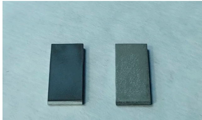
Figure 2. Photographic image of fresh superhydrophilic sample (left) and superhydrophilic sample after 53 thermal cycles (right).
