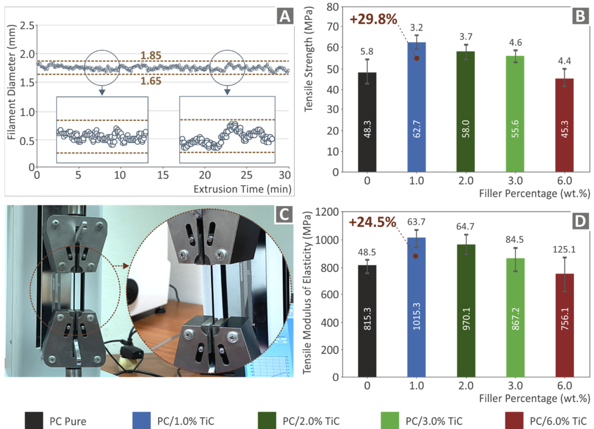
Figure 6. (A) Real-time diameter measurement of the produced filament during the filament extrusion process, (B) mean tensile strength values and deviation of the produced filament for all materials studied, (C) experimental setup for the produced filament tensile tests, and (D) mean tensile modulus of elasticity values and deviation of the produced filament for all materials studied.
