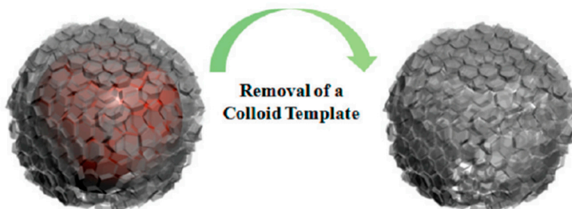
Figure 3. Schematic representation of rGO hollow capsules assembly. Republished with permission from Ref. [3]. Copyright 2022 American Chemical Society.
