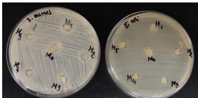
Figure 10. M 0 = PVA/XG-100/0; M 1 = PVA/XG-90/10; M 2 = PVA/XG-80/20; M 3 = PVA/XG-70/30; M 4 = PVA/XG-60/40; M 5 = PVA/XG-50/50.
