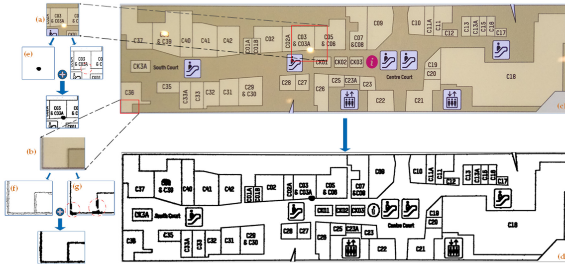
Figure 5. The preprocessing result is presented: (a,b) represent a partial enlarged view taken from F_0 , (c) denotes the shopping mall plan F_0 , (d) denotes the preprocessing result F_1 , (e) denotes the result of exposure point detection F_{b2} , (f) denotes the result of canny edge detection F_{b3} , and (g) denotes the result of adaptive threshold segmentation F_{b1} .
