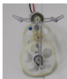
(b) Assembly part for base, gear, and linkage of original MAV (aluminum)
