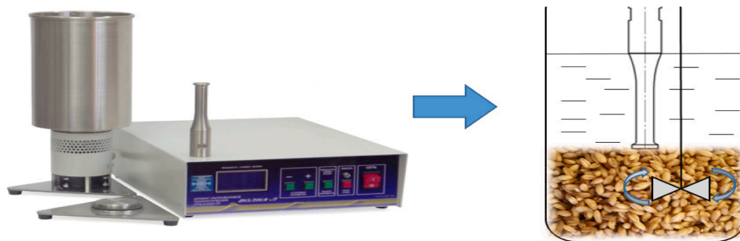
Fig. 2. The ultrasonic vibrating system.
