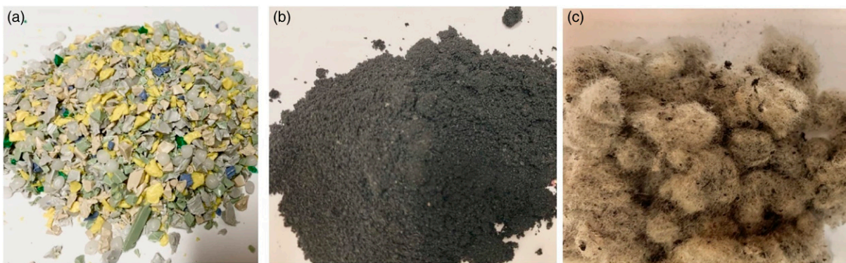
Figure 1. General view of: (a) rHDPE flakes, (b) RR particles, and (c) RTF as received. rHDPE: recycled high density polyethylene; RTF: recycled tire textile fiber.
