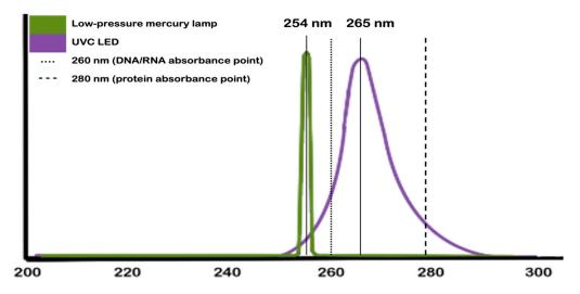
**Figure 1.** Wavelength peaks according to the UVC sources. Note: We abstained from providing the curve for medium-pressure lamps because they overlap with one of the UVC LEDs. For technical parameters about UVC traditional sources and LEDs, we suggest moving to Section 4.
