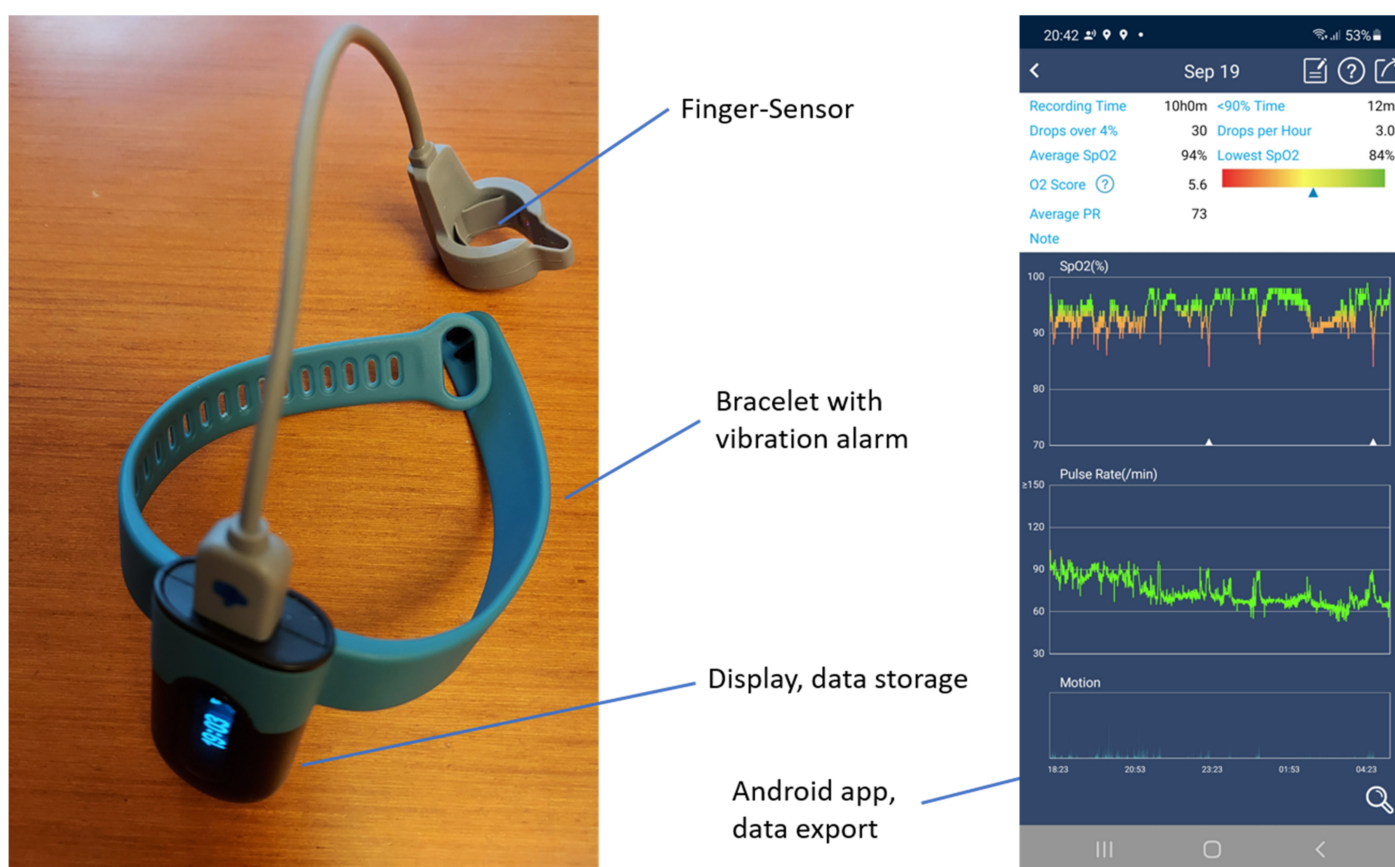
Figure 1. A picture of the device and a screenshot of the data evaluation in the android app.
