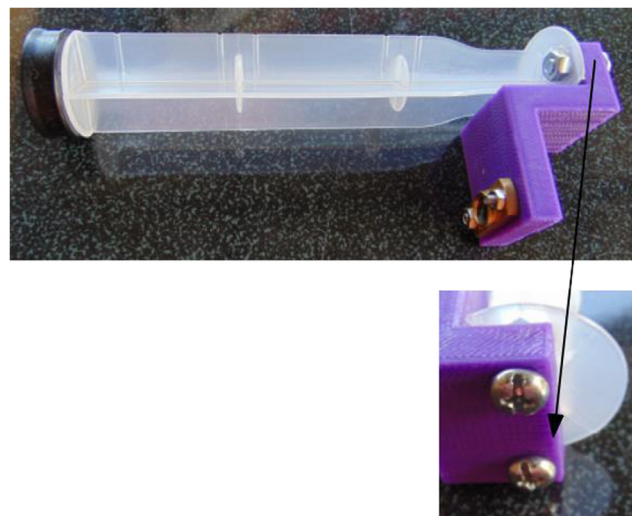
Fig. 9. Plunger attached to its holder.
