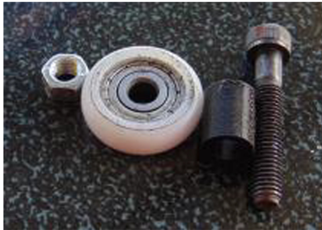
Fig. 6. Wheel set to make the sliding motor carriers on axes X and Y.
