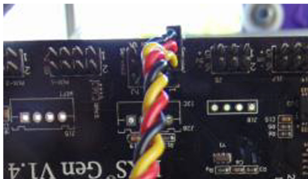
Fig. 26. Servo cable connected to the control board.
