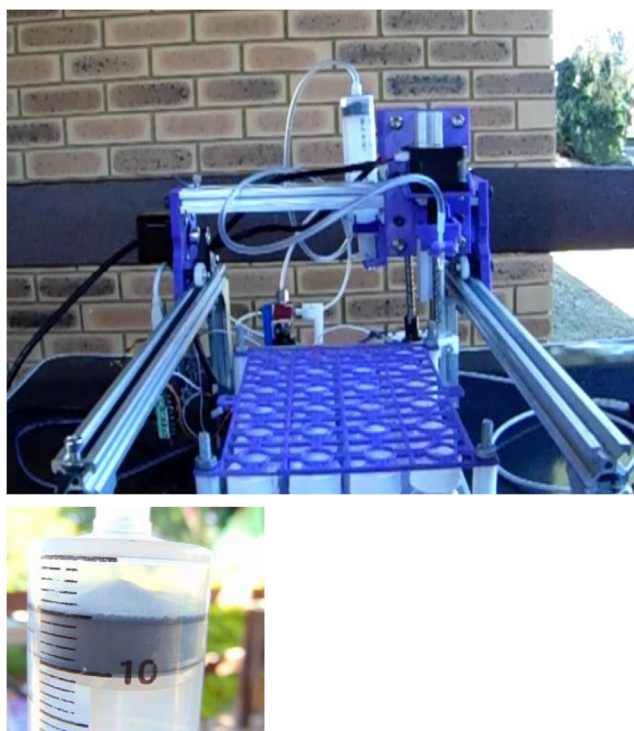
Fig. 34. Initial positions for X, Y, Z and E axes. Below: detail of the plunger at its top position.
