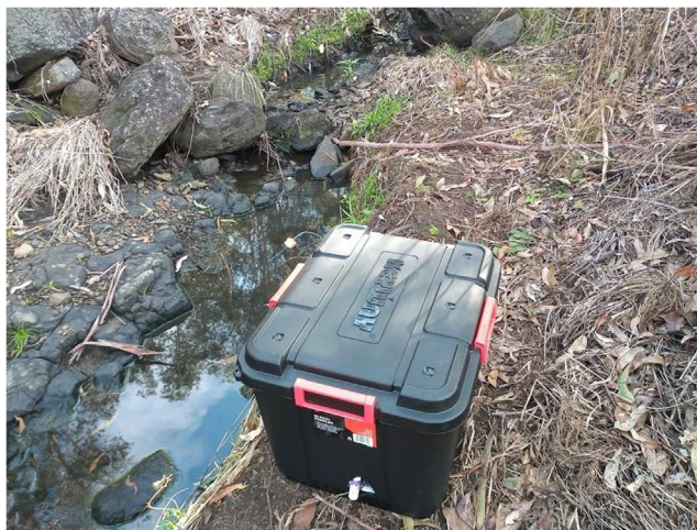
Fig. 38. Autosampler close to a small creek in the Southern Cross University campus.
