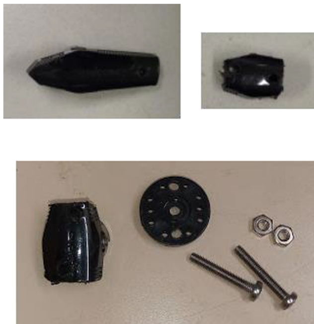
Fig. 24. Modifying the valve and servo levers.
