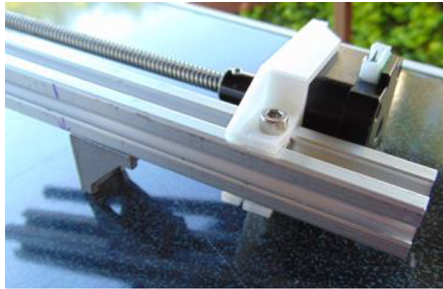
Fig. 4. Motor mount attached to 200 mm extrusion profile.
