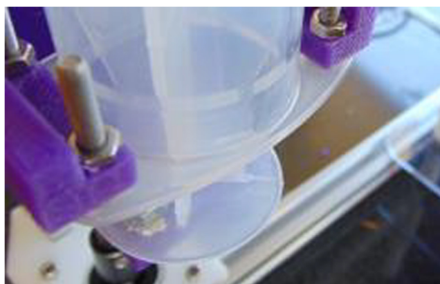
Fig. 11. Syringe attached to E axis syringe holder.
