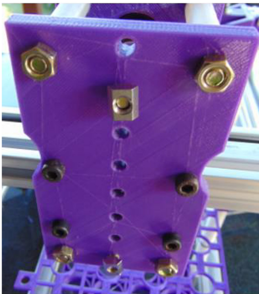
Fig. 19. X axis connected to the Y axis plates.
