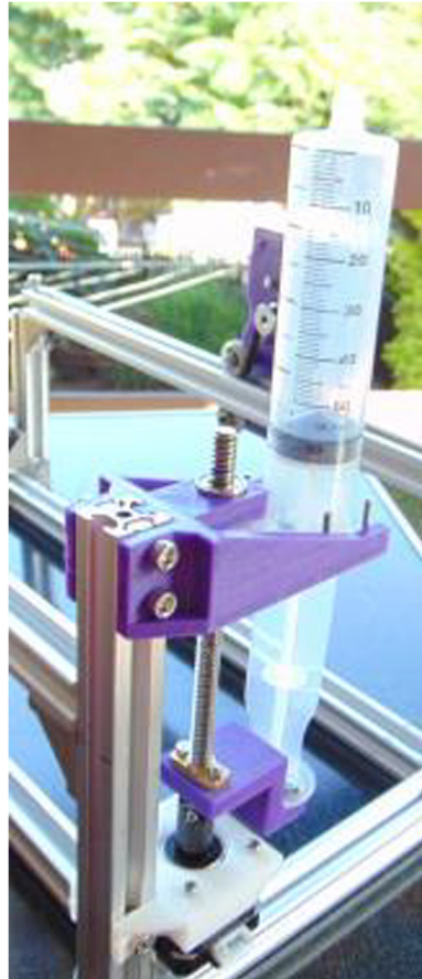
Fig. 12. Syringe attached to the E axis.
