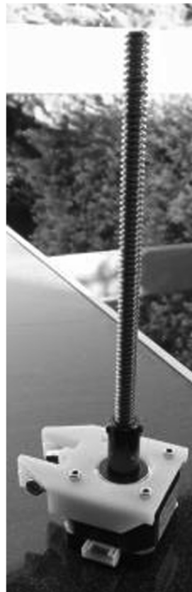
Fig. 3. E axis motor with its lead screw connected using a shaft coupler.
