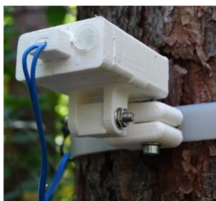
Fig. 4. Tree response sensor (TRS) mounted to the stem of a Scots pine tree.
