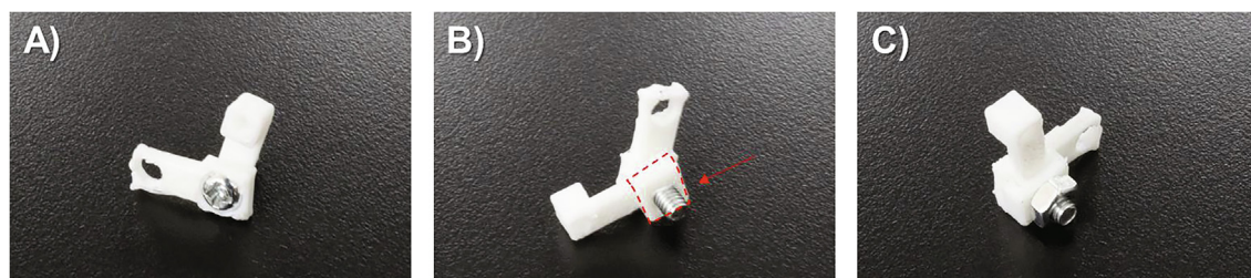
Fig. 7. Wheel height adjustment unit. A) arm_1 and arm_2 connected by a screw. B) Screw is held in place by using arm_fastener (indicated with red box and red arrow). C) Pieces are fastened by using an M4 nut. (For interpretation of the references to colour in this figure legend, the reader is referred to the web version of this article.)
