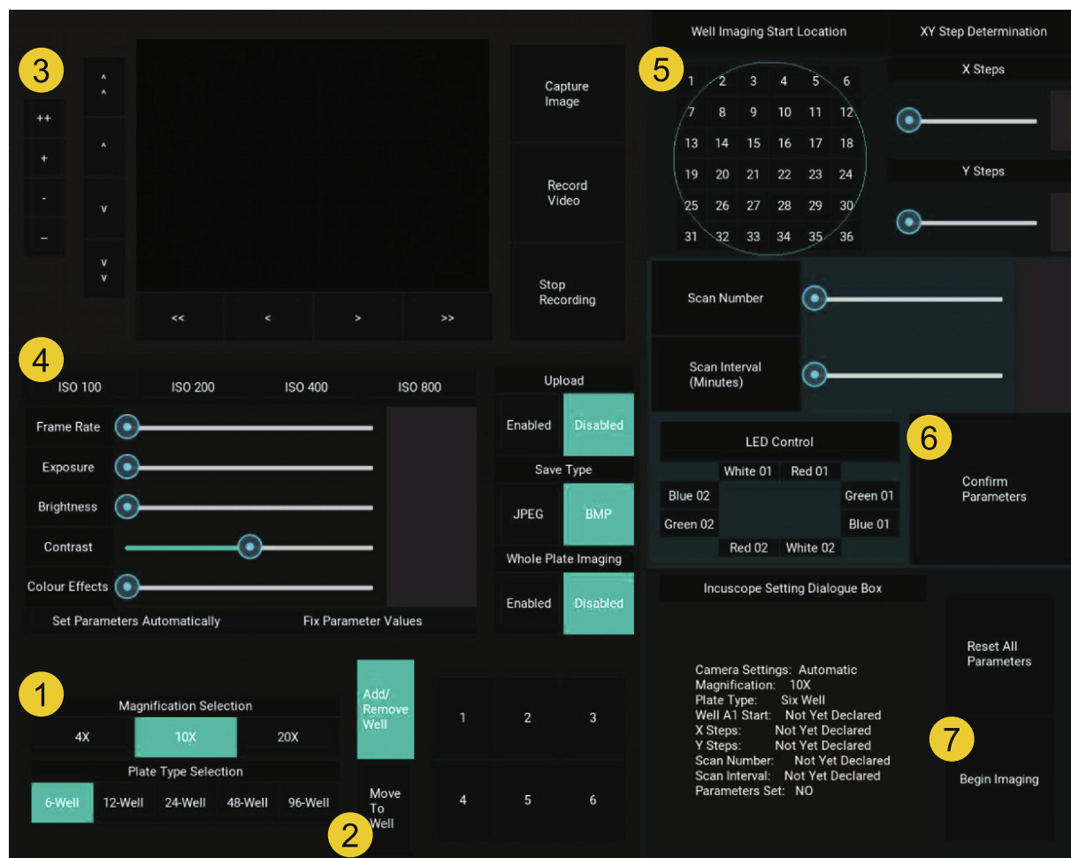
Fig. 12. Quick-Start Operational Guide to Routine Use of the Incubot GUI. 1) Select your hardware settings (magnification and plate type). 2) Select the “Move to Well” button and select a well of your choice from the grid layout to the right of it. 3) Adjust the X and Y positions until cells are in view and adjust the Z position until cells are in focus. 4) Adjust the image acquisition parameters if needed and alter any image acquisition parameters you wish to. 5) Select an appropriate start location for your experiment and select the number of images in the X and Y axes you wish to collect. Alter the scan number and scan interval parameters to suit your experimental needs. 6) Once all settings are to your liking, confirm the parameters by pressing the “Confirm Parameters” button. 7) Once sure that imaging is established to your liking, press the “Begin Imaging” button to begin the process of imaging. The Incubot will be unresponsive during the imaging run, so if emergency stopping is required, the Pi must be physically switched off and back on again. Note that this will result in the loss of positional XYZ information and the Incubot will assume the position it is left in is X0Y0Z0. You may need to manually move the Incubot to its X0Y0, or via the Arduino IDE once rebooted using negative X and Y coordinates.
