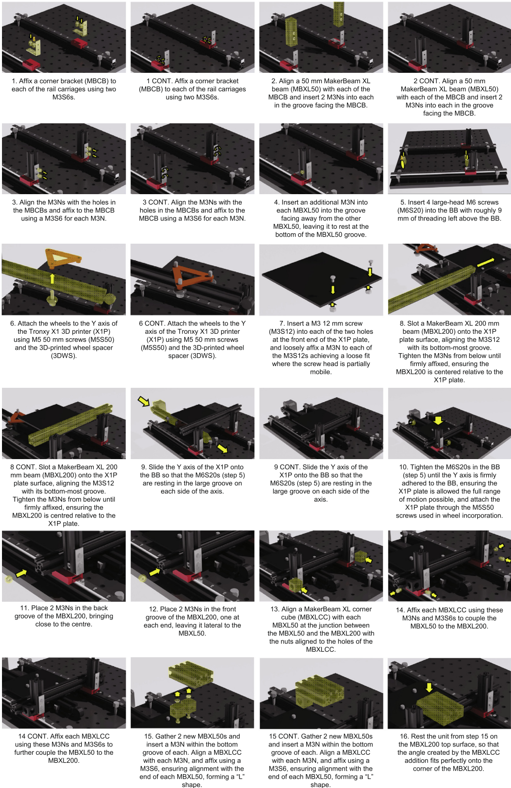
Fig. 3. Incubot Assembly Visual Guide – Axes Coupling Part I.
