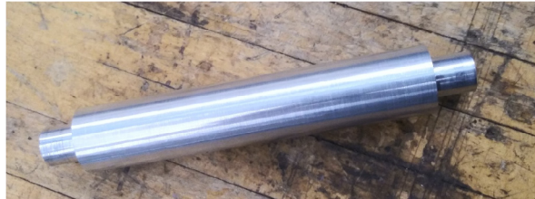
Fig. 3. Machined drive roller, cut on a CNC lathe.
