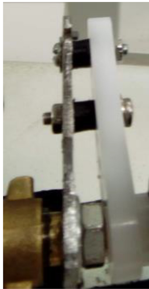
Fig. 15. Valve lever connected to servo arm. Notice screws connected at opposing orientations.
