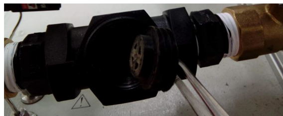
Fig. 18. Sieve to be placed inside the T piece to avoid samples to settle at the perpendicular connection.
