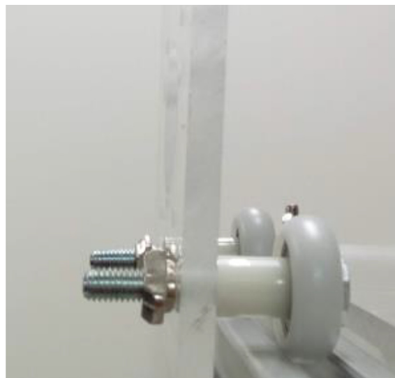
Fig. 5. Wheels fixed to the one of the acrylic supports.
