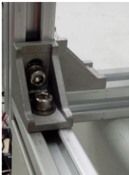
Fig. 10. Bracket (2028) connecting extrusion profiles. Notice M5 screws and washers. Hammer nuts are inside the extrusion profile grooves.
