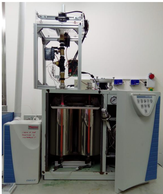
Fig. 1. EA autosampler mounted on top of an elemental analyzer. The sample table is the four-legged acrylic sheet supporting the carousel. The purging pipe is the pipe beneath the sampling table and connected to the elemental analyzer.
