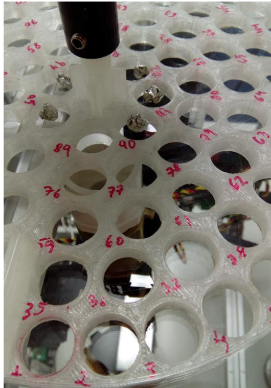
Fig. 4. Carousel made of clear PLA, allowing writing of the sample positions with a pen.
