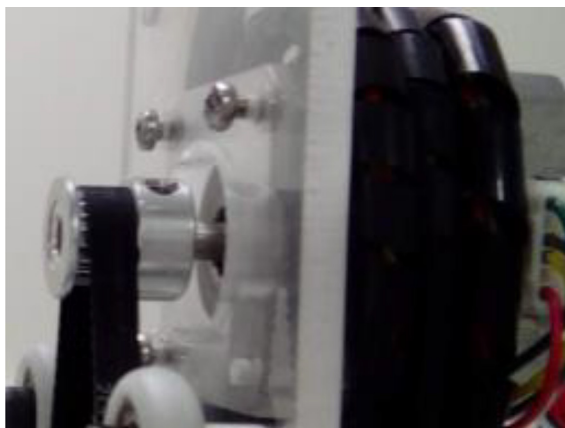
Fig. 6. Stepper motor fixed to one of the acrylic supports. Here only 3 screws are holding the motor.
