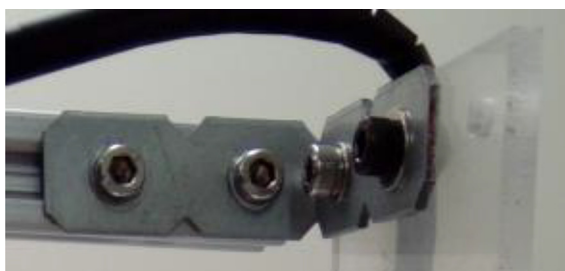
Fig. 7. Bracket fixed to acrylic support.
