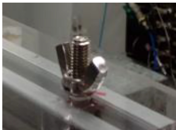
Fig. 11. Acrylic sheet connected to extrusion profile using hammer-head screw and wingnut.
