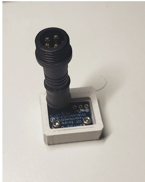
Fig. 14. SHT31D screwed into its case.
