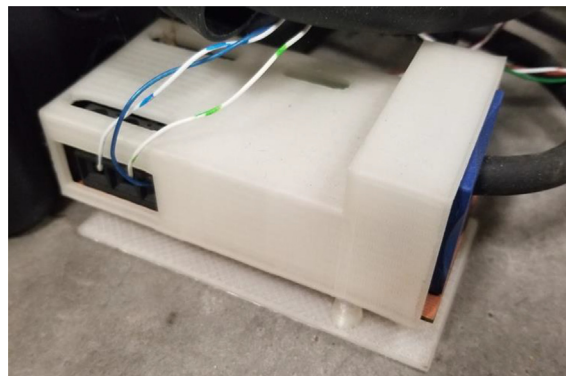
Fig. 5. PLA casing covering voltage and current circuit attached around welding electrode constructed from Pinar et al. [30].
