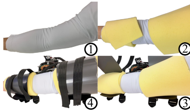
Fig. 13. Instructions for donning the exoskeleton, in order counter-clockwise. First, a sleeve is put on the wearer, followed by wrapping the arm in foam. Next, the exoskeleton is wrapped around the foam, and the straps tightened.
