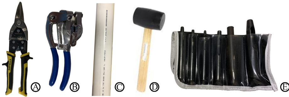
Fig. 3. Primary hand tools for fabricating the frame. These include: (A) FMHT73756 tin snips, ($16–18) – used to cut H1, a long thin beam, into shorter pieces; (B) Metal Hand Punch ($25–39) – used to punch holes in beams; (C) PVC Pipe ($3–10) and (D) Rubber Mallet ($2–10) – used to bend the aluminum braces into the curved arm shape; and (E) Hollow Punch Tool ($10–20) – creating mounting holes in fabric. Additional required equipment not shown above are: screw drivers, a sewing machine, a soldering iron, a table mount, and a power supply (or a battery).
