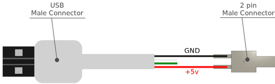
Fig. 5. External power supply cable made with a USB cord.
