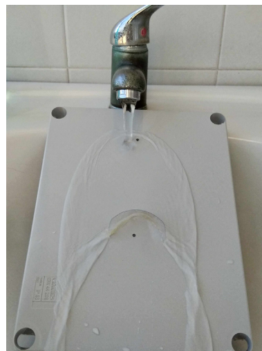
Fig. 19. A simple test to prove the effectiveness of hoods obtained by cutting strips from recycled plastic bottles and fixed through hot glue on the enclosure lid.
