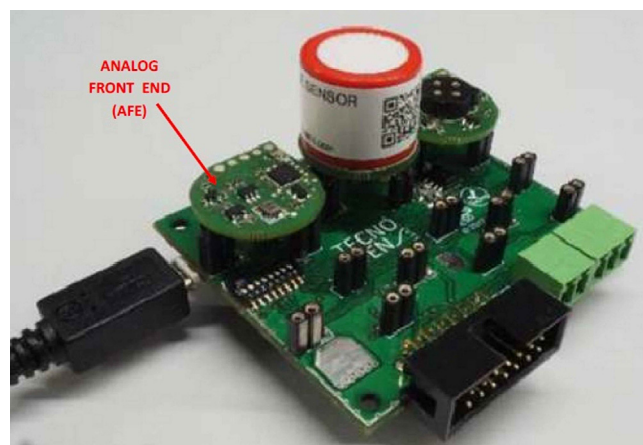
Fig. 10. The Multisensor board by Tecnosens (dimensions: 6,5cm × 6,3cm). Each type of sensor must be connected through the AFE adapter (not supplied with the Multisensor board). The sensor adapters must be purchased apart from Tecnosens.
