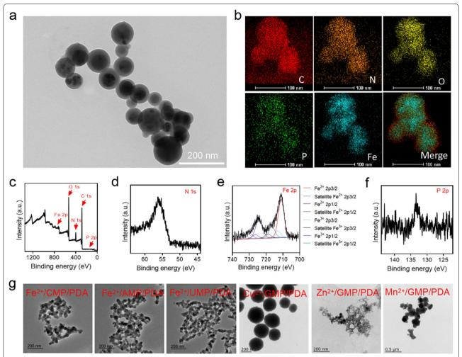
Fig. 1 Characterization of FeGPNPs based on metal and nucleotide coordination. a TEM image of FeGPNPs. b EDX mapping of FeGPNPs. c Survey XPS spectrum of FeGPNPs. d—f High-resolution XPS spectra of N 1s, Fe 2p, and P 2p, respectively. g TEM images of nanoparticles obtained using different metal ions and nucleotides
