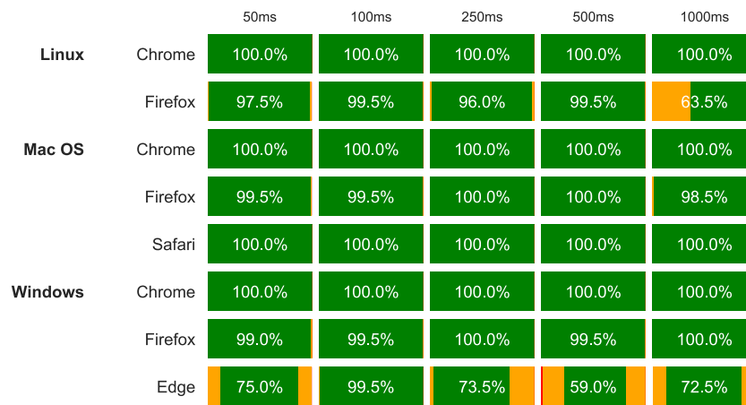
Fig. 10 Timing validation results for stimulus presentation, in percent of target frames hit across simulated durations, browsers, and systems. The green areas represent the proportion of exact matches, orange areas are one frame to early or to late, and red areas two frames or more (only the case for Internet Explorer Edge, in less than 1% of the two longest presentation intervals). See also https://lab.js.org/performance for the most recent timing results
