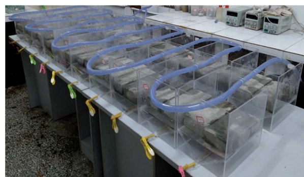
Fig. 2 Experimental rainfall simulation device in operation.
