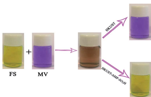
Fig. 4 The reverse performance of HKUST and HKUST-AMP-SO 3 H for FS–MV mixture.
