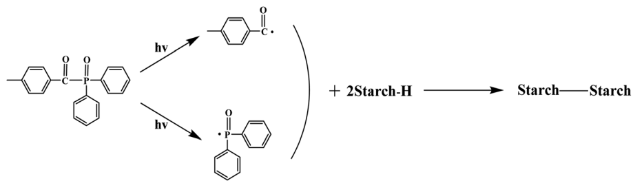
Fig. 3 Mechanism of TPO decomposition and cross-linking between starch macromolecules.
