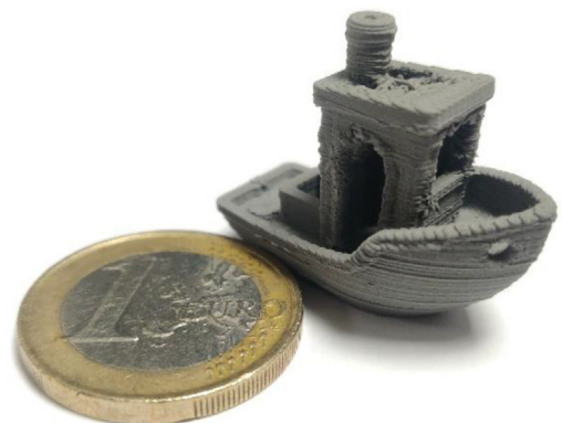
Fig. 32. Benchy test print (green piece) and tensile specimens (sintered) for micro-tomography printed with a 0.25 mm diameter nozzle. (For interpretation of the references to colour in this figure legend, the reader is referred to the web version of this article.)
