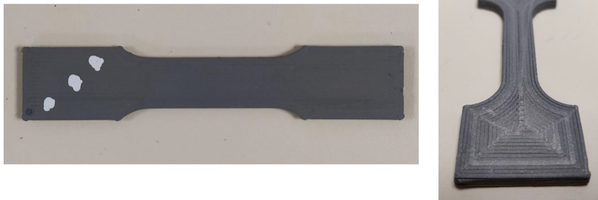
Fig. 34. Tensile test piece. Green part on the left and sintered part on the right.
