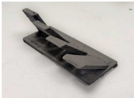
Fig. 31. Test part of the printable inclination without support (30°, 40°, 50°, 60°) (green part).
