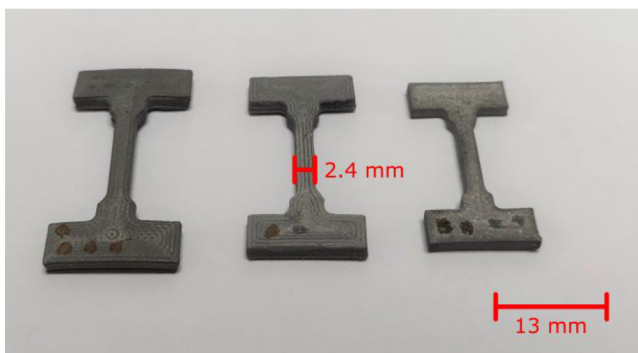
Fig. 32. Benchy test print (green piece) and tensile specimens (sintered) for micro-tomography printed with a 0.25 mm diameter nozzle. (For interpretation of the references to colour in this figure legend, the reader is referred to the web version of this article.)
