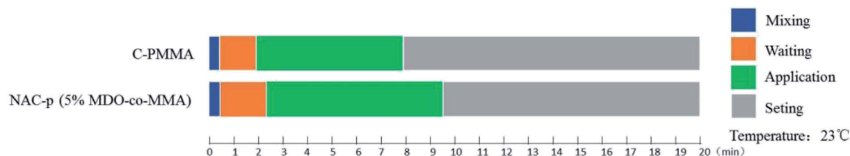
Fig. 2 Solidification characteristics of NAC-p (5% MDO-co-MMA). Measured at 23 °C with C-PMMA as a control.
