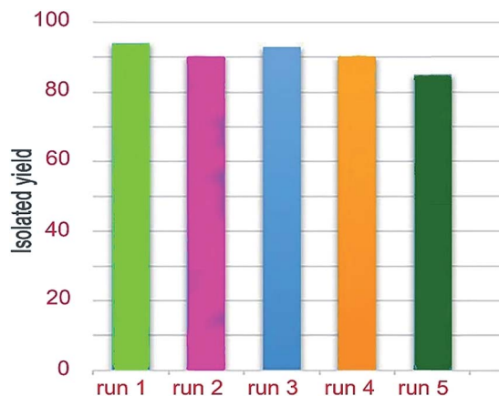
Fig. 9 Recyclability study of the nanocatalyst, W(IV)/NNBIA-SBA-15, for the reaction of isatin (1 mmol), malononitrile (1 mmol) and hydantoin (1 mmol) under optimized conditions.
