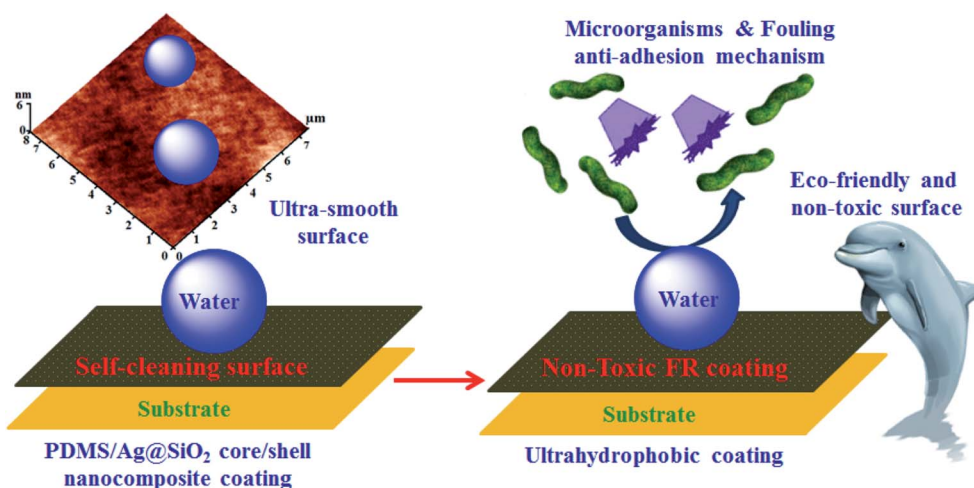
Scheme 2 Non-toxic ultrahydrophobic surface of PDMS/spherical Ag@SiO 2 core-shell FR nanocomposites behaviour and their failure adhesion mechanism.
