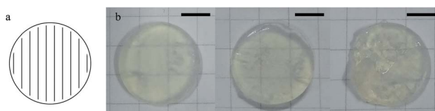
Fig. 3 (a) Illustration of the scan path for a cycloidal pattern (the red line represents the hatch distance), (b) photos of the green parts (cylinder with diameters of 14 mm and thicknesses of 1.4 mm) fabricated under different SL parameters (from left to right, 60 mW 46 \text{mm s}^{-1} , 130 mW 100 \text{mm s}^{-1} and 200 mW 154 \text{mm s}^{-1} , scale bar, 2.5 mm).
