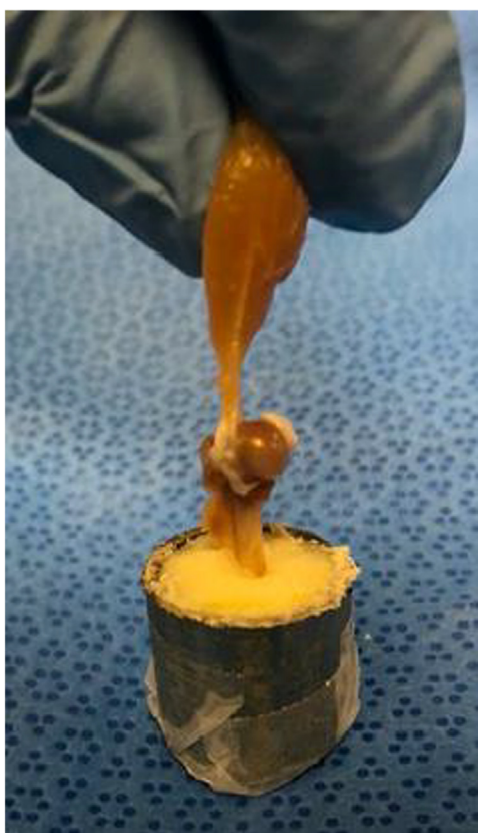
Figure 2 The muscle-tendon-bone specimen potted for biomechanical testing.
