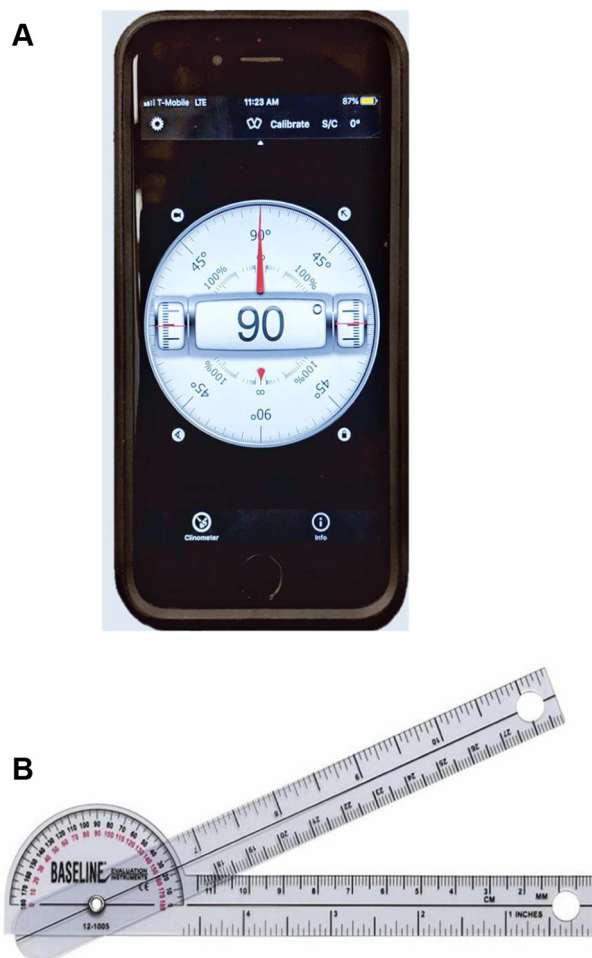
Figure 1 (A) Clinometer application on the iPhone, (B) Standard half-circle goniometer used to measure forearm ROM.
