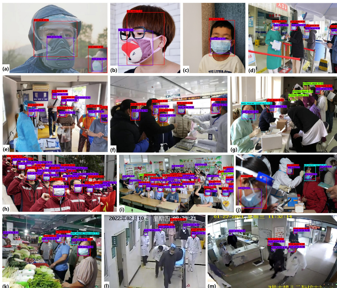
Fig. 15. The detection results of SMD-YOLO detector with real-world face masks wearing status under the various environments. (a)(b)(c) On medium individual faces with a distinctive mask. (d)(e) At the entrance of the hospitals. (f)(g) When small queuing or registering in a small scale at the hospitals. (h)(i) In the densely crowded public areas indoors and outdoors. (j)(k) In the nighttime environment. (l)(m) Inside the hospital corridor from the camera of monitor.
