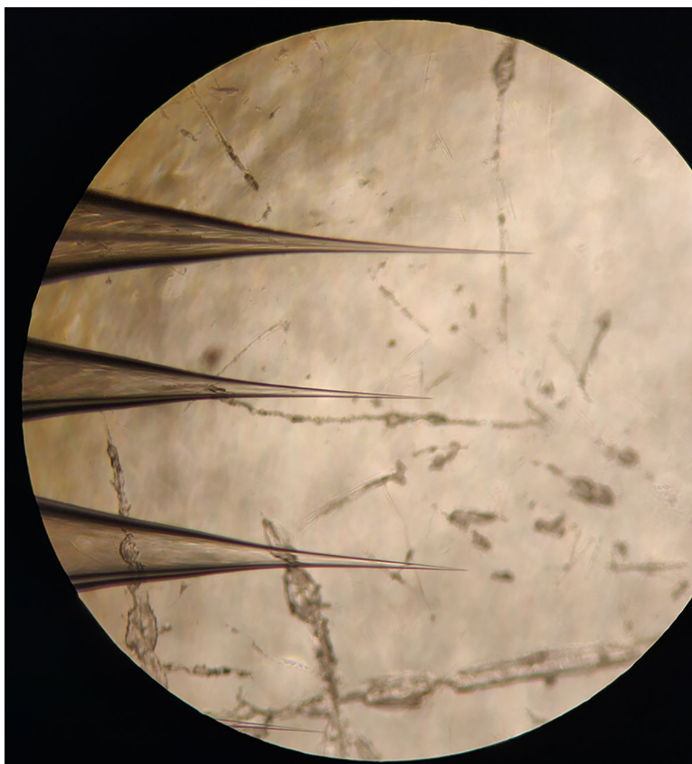
Figure 1. Four-fold magnification of the tips of emitters. The general tip shape of nano electrospray ionization emitters that work well at the spray voltages specified in Table
