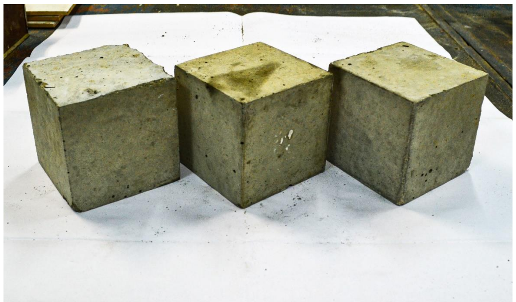
Figure 1. Samples of nano-modified micro silica heavy concrete for compression testing.
