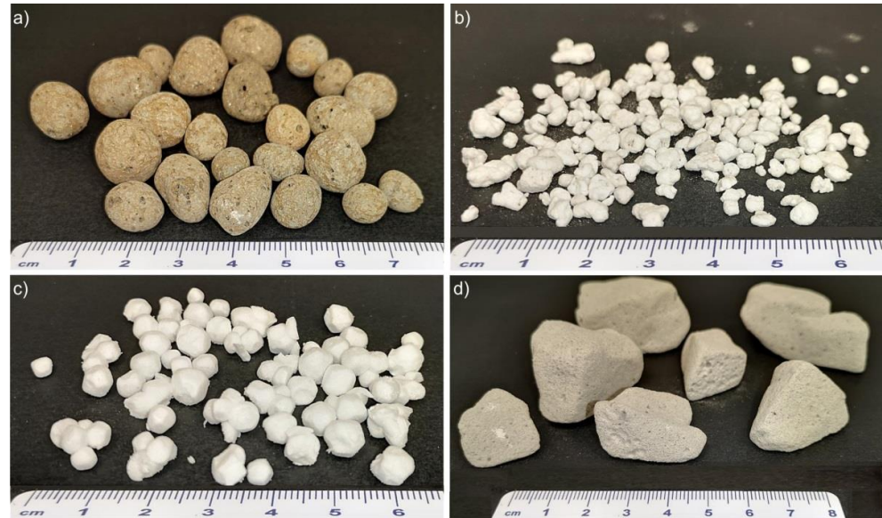
Figure 1. Photographs of the applied LWAs: (a) expanded clay, (b) perlite, (c) expanded polystyrene and (d) expanded glass.
