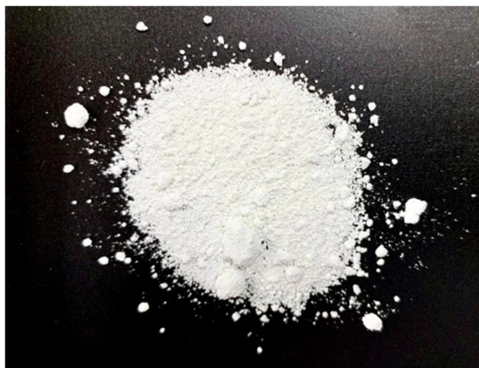
Figure 1. Reagent-grade \text{TiO}_2 powder (anatase, 99% purity).
