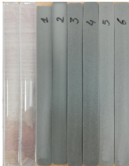
Figure 4. Experimental samples prepared for tensile tests, following ISO 6721 standard requirements. From the left: pure silicone samples; 1 and 2—0.8 mmol/g multilayer silicone composites samples; 3 and 4—1.6 mmol/g multilayer silicone composites samples; 5 and 6—3.2 mmol/g multilayer silicone composites samples.
