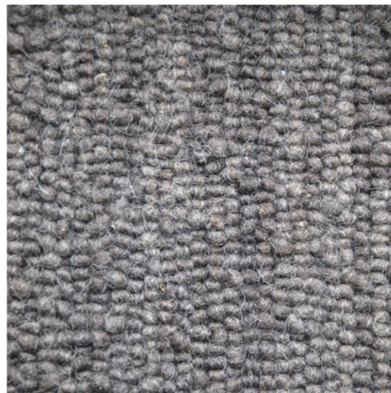
Figure 6. Tufted fabrics manufactured from core rug yarn.
