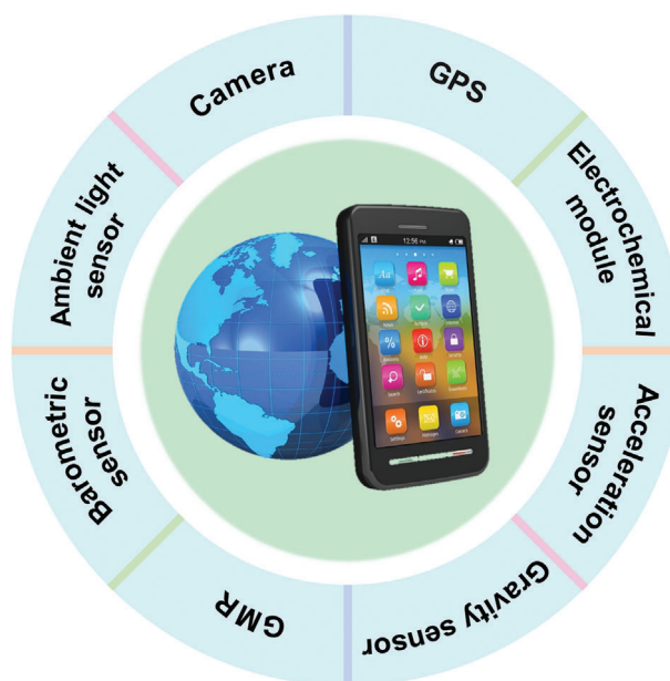
Figure 5. Built-in functional modules in smartphones include the camera, ambient light sensor, distance sensor, gravity sensor, acceleration sensor, electrochemical module, magnetic sensor, barometric sensor, gyroscopes, global position system (GPS).
