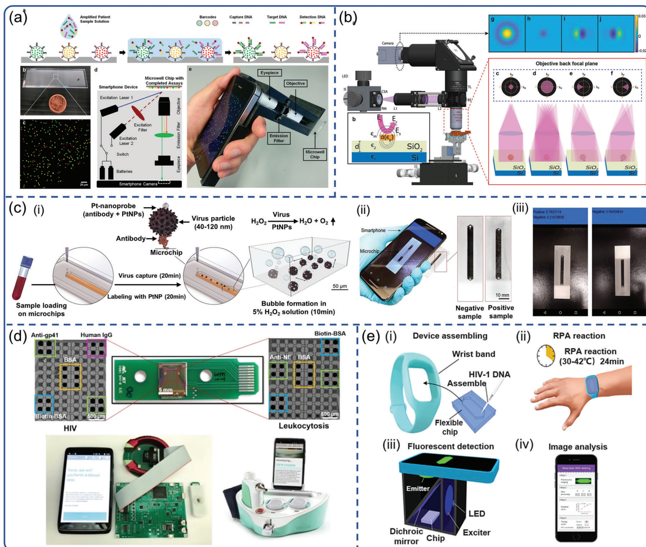
Figure 9. a,b) Smartphone-based microscopy for virus disease diagnostics. a) Overview of the smartphone-based microscopy utilizing quantum dot barcodes. The assay involves the addition of patient samples to a chip coated with microbeads and related optical principles. Reproduced with permission. [149] Copyright 2015, American Chemical Society. b) SPIR microscopy and schematic of the experimental setup. Reproduced with permission. [150] Copyright 2018, American Chemical Society. c–e) Smartphone integrated with other types of biosensors for virus disease diagnostics. c) 3D schematic of the CNN-nanoparticle-enabled smartphone for virus detection. Reproduced with permission. [152] Copyright 2020, American Association for the Advancement of Science (AAAS). d) Image of GMR nanosensor chip on PCB, and essential components of the redesigned Eigen diagnosis platform. Reproduced with permission. [153] Copyright 2019, Elsevier. e) Wearable RPA sensing system for rapid detection of HIV-1 DNA is consisted of a fluorescence image box and PDMS-based flexible chips. Reproduced with permission. [155] Copyright 2019, Elsevier.
