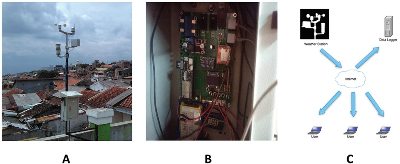
Fig. 2. A) AWS, the weather station, complete modules; B) microcontroller with a low power co-processor, additional external memory (SDCard), GPS and GSM modules; C) logger system for data collection and storage system.
