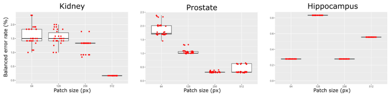
Figure 3: Prediction error variability for the classification task trained on the tissue types separately. Hippocampus classifier showed best accuracy, followed by prostate and kidney. The relationship between patch size and classification error can be observed: bigger patches seem to have lower error rates.
