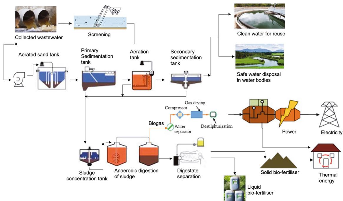
Figure 9. Conventional Wastewater Treatment Plant integrated with operational AD system for biogas production and electricity generation.
