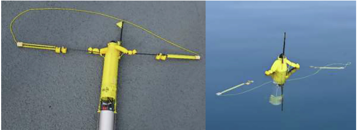
Fig. 8. Pick-up arms and wire system for instrument retrieval (left) and wire system position in water (right). The yellow wire is attached to the pressure hull and forms a closed loop that runs through the pick-up arms. Photo courtesy of Peter Bondo Christensen. (For interpretation of the references to colour in this figure legend, the reader is referred to the web version of this article.)
