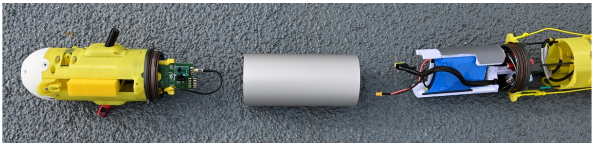
Fig. 20. The disassembled profiler before preparing for deployment. From left to right: Bottom hull, pressure hull and top hull. Photo courtesy of Peter Bondo Christensen.
