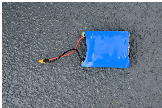
Fig. 9. The complete battery pack covered in heat shrink tubing. Photo courtesy of Peter Bondo Christensen.
