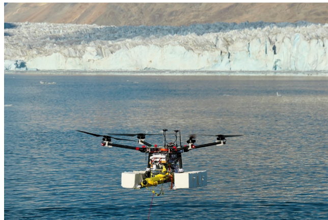
Fig. 2. ARC-TOP mounted on UAV during testing in Isfjord in NE Greenland. Photo courtesy of Søren Rysgaard.
