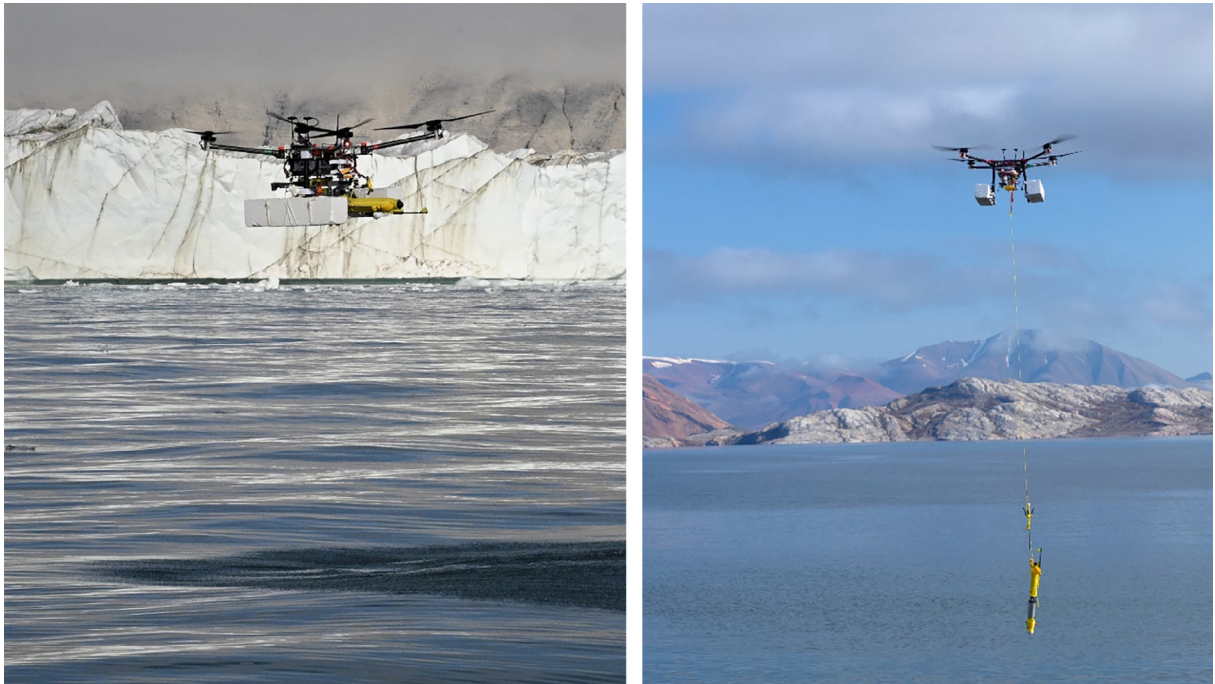
Fig. 25. Profiler delivery just prior to deployment (left), photo courtesy of Peter Bondo Christensen., and profiler retrieval after deployment (right), photo courtesy of Nils Risgaard-Petersen.
