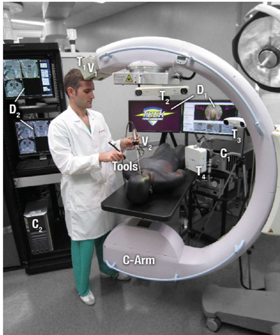
Fig. 1. Prototype C-arm for CBCT, tracking and navigation technologies. Systems labeled in the photograph include the C-arm, tracked tools, T1 (MicronTracker, Claron , Toronto ON), T2 (Polaris Spectra, NDI , Waterloo ON), T3 (Polaris Vicra , NDI ), T4 (Aurora, NDI ), V1 (MicronTracker, Claron ), V2 (Video endoscope, 7230AA, Karl Storz , Tuttlingen Germany), C1 (TREK navigation workstation), C2 (C-arm image acquisition workstation), D1 (TREK navigation displays), and D2 (C-arm image displays). C2/D2 are traditionally separate from the tableside setup, operated by a technologist to acquire and process C-arm images and optionally exposed to the surgeon for image review. Instead, images from C2/D2 are acquired by the technologist and transferred to C1/D1 for real-time guidance and visualization by the surgeon
