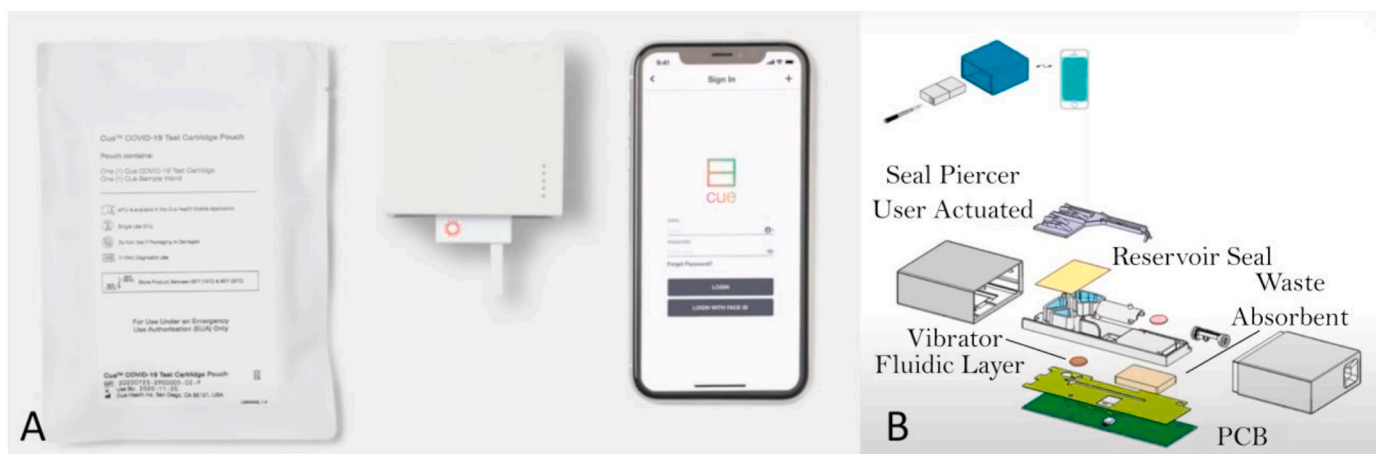
Fig. 3. A) The Cue COVID-19 Test from Cue Health Inc. with a cartridge pouch, the reader (with a cartridge with a sample wand inserted) and the app. Picture taken from: https://www.cuehealth.com/products/how-cue-detects-covid-19/ . B) Exploded view of the test cartridge and the Cue Cartridge Reader (Sagentia Innovation, 2021).
