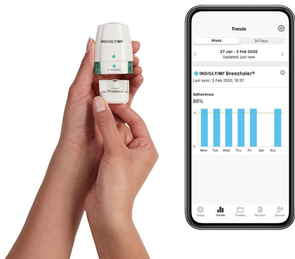
Fig. 1 The Breezhaler® device with the Propeller Health® sensor and smartphone app. Image © Propeller Health
